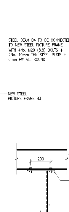
DETAIL C STEEL BEAM TO SHS INTERNAL COLUMN CONNECTION DETAIL (Scale 1:10)
